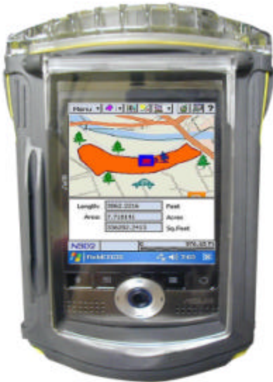
PDA with high-performance GPS in waterproof case
