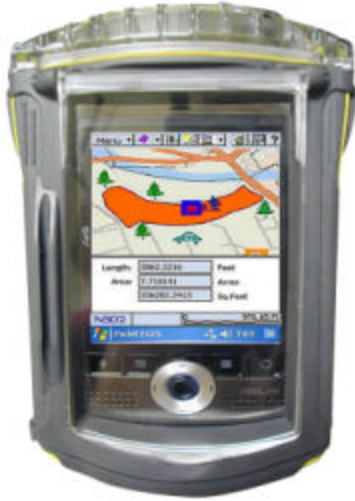
PDA with high-performance GPS in waterproof case
